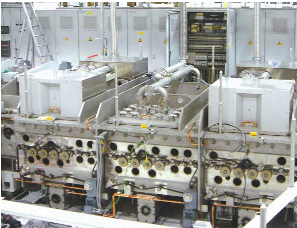
滚动驱动用于真空镀膜 Roller drive for vacuum coatings Complete drive system suitable for special requirements in vacuum coating applications. 完整驱动系统适合于特殊要求的真空镀膜应用
