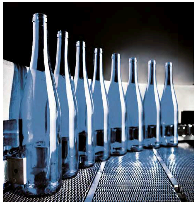
Cross conveyor at the cooling furnace 冷却炉的横式输送机
