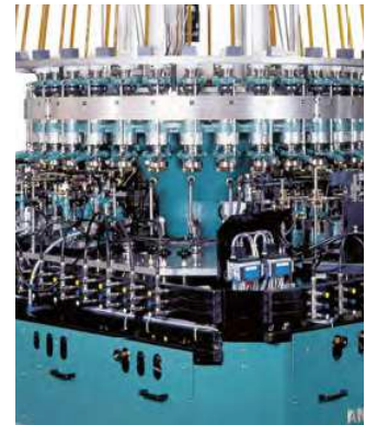
医药玻璃器皿 Medical glassware A single Biflex inverted tooth chain is used for the synchronous rotation of all 32 forms in a forming glass lathe for processing glass vials. 单个Biflex齿形链用于玻璃车床加工玻璃小瓶的所有同步旋转32道成型流程。
