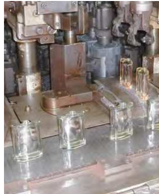
小型玻璃产品的特殊版本 Special version for small glass products Individually adapted inverted tooth conveyor chains for a flask production line. 单独适应齿形输送链用于烧瓶生产线
