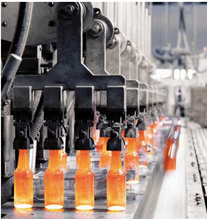
Machine conveyor on IS-machines IS-机器输送机
