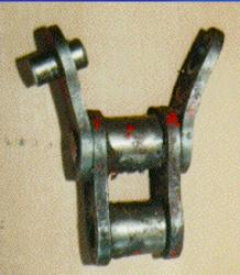
Look for evidence of deformed material. The chain plate in the top image has failed in overload
