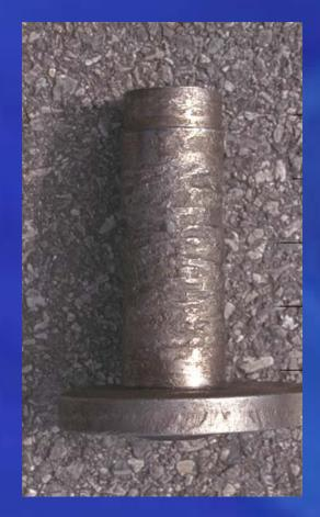
Lack of lubrication or excessively high running loads
