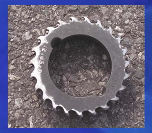
This sprocket has run with poor lubrication in a dusty environment.
