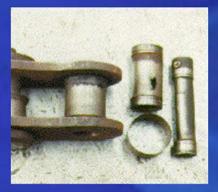
In very harsh conditions a combination of water and corrosive chemicals can caused havoc.
